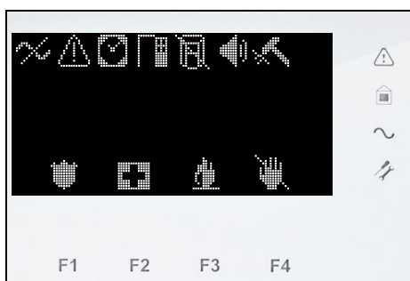
Figure 4 - KP500DP/N - KP500D/ST keypad display and status icons
