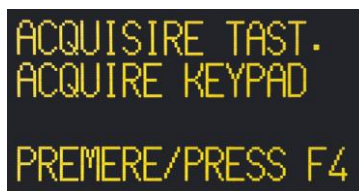
Figure 64 - Message of KP500DP/N - KP500D/ST keypad acquisition
